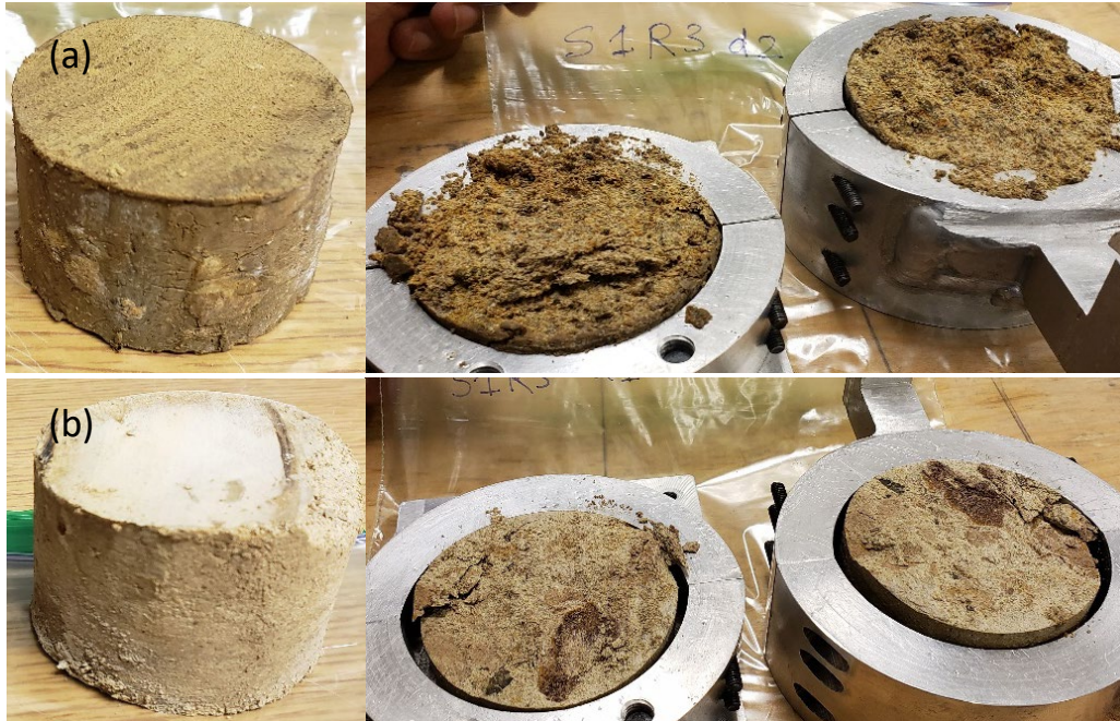
Figure 10: Specimen before and after shearing: (a) low suction; (b) high suction
