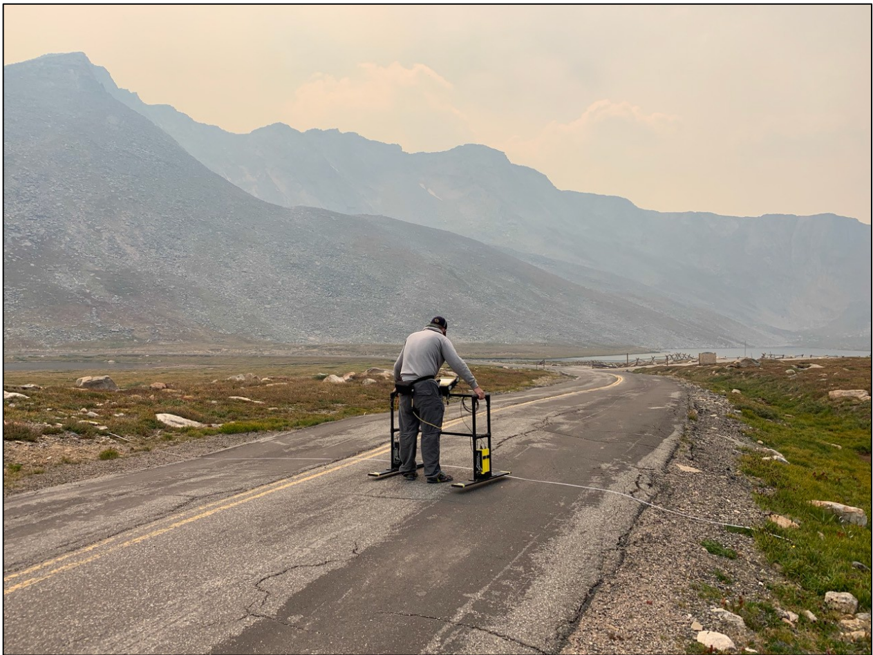
R. Bonnell conducting 100 MHz common offset ground-penetrating radar surveys near Summit Lake, Mt. Evans.
