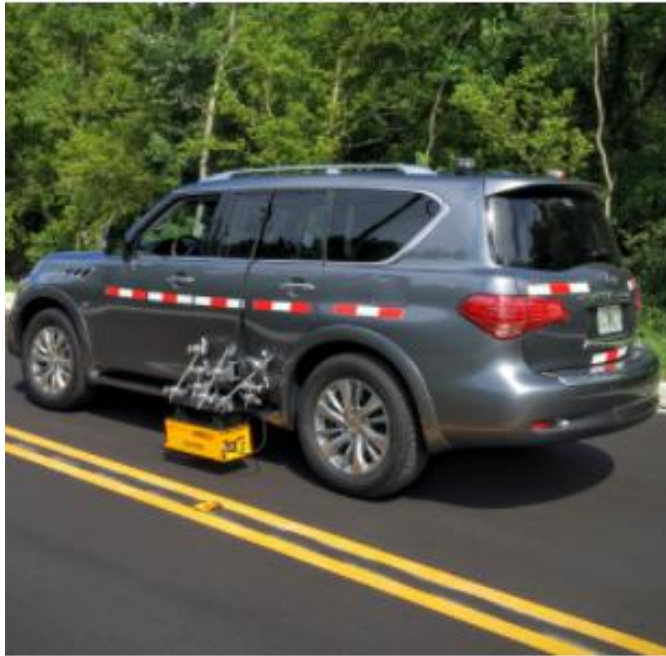
Figure 1. Mobile retroreflectometer system.
