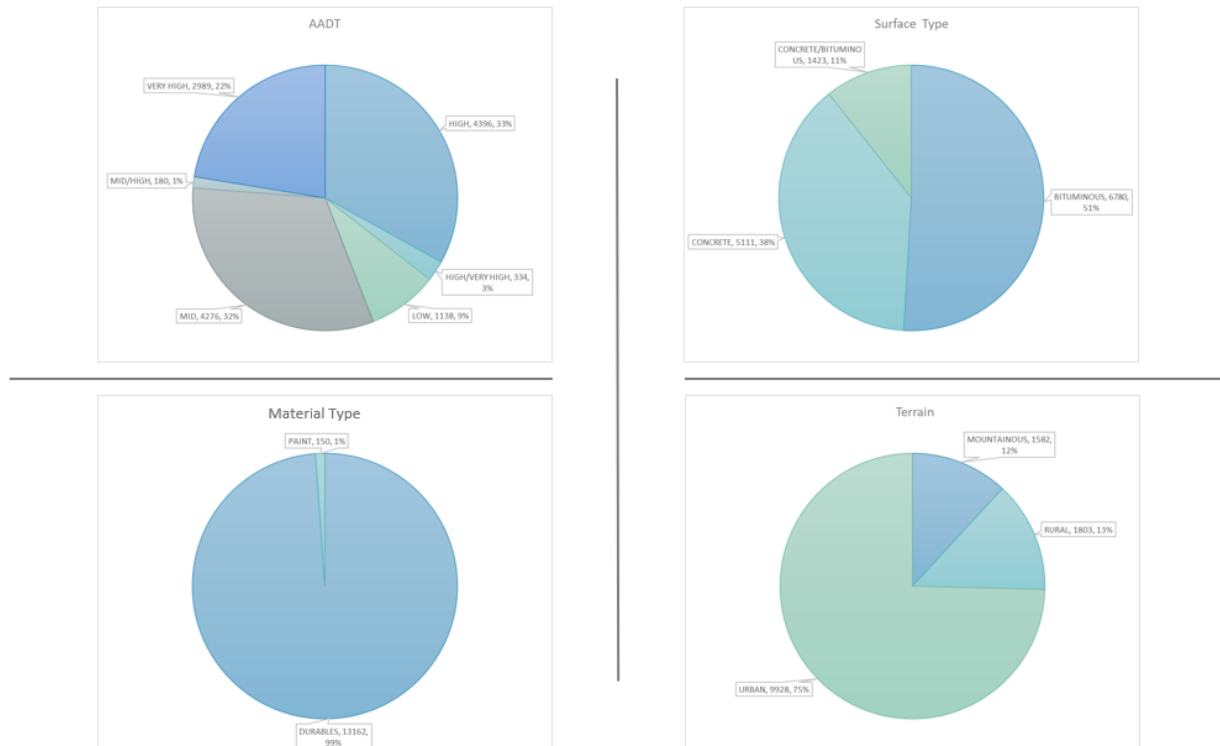
Figure 11. Road feature surveyed in Region 1 for AADT, Surface Type, Material Type and Terrain. In each inserted figure, the callout indicates feature, total mileage, and percentage.
