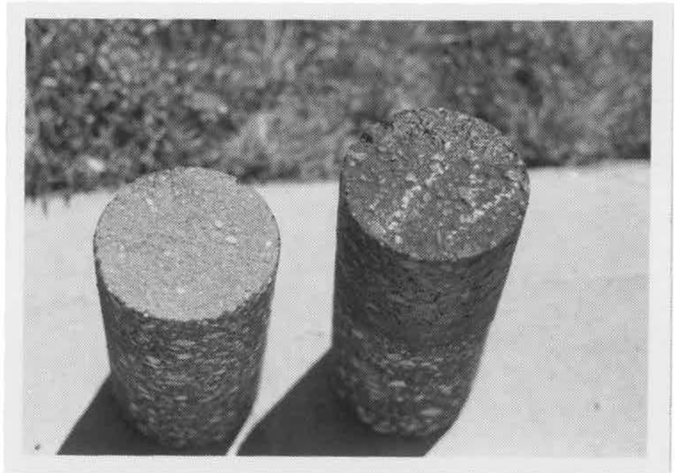
(W) core with pits from dissolved Verglimit
