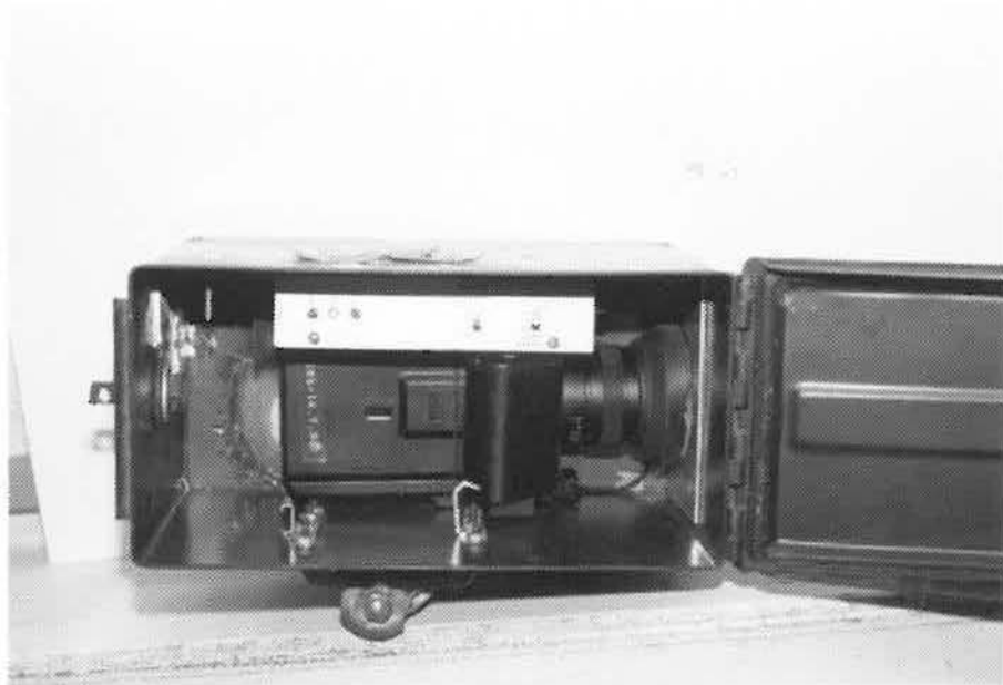
(N) Camera, timer, and battery pack mounted in an ammo can
