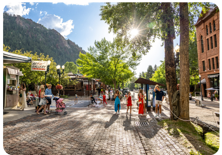
A downtown streetscape in Aspen uses street trees and permeable pavement, two forms of green infrastructure.
