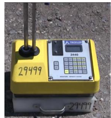
T-310 Figure 4: Standardizing the Nuclear Density Gage
