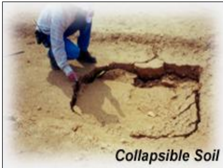
Figure 28: Sinkhole development as a result of collapsible soil deposits settling at depth.
