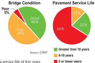
**Pavement conditions need improvement** as 66% of the region's pavement has a service life of five years or less. Service life is a calculation based on a combination of age and expected design life of pavement. With maintenance and minimal treatments, pavement life can be extended. CDOT is currently exploring enhanced road-management methods including new preservation strategies to maintain the highest roadway surface grades possible, despite declining revenues.
