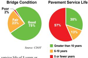
**Pavement conditions need improvement** as 57% of the region's pavement has a service life of 5 years or less. Service Life is a calculation based on a combination of age and expected design life of pavement. With maintenance and minimal treatments, pavement life can be extended. CDOT is currently exploring enhanced road-management methods, including new preservation strategies, to maintain the highest roadway surface grades possible, despite declining revenues.
