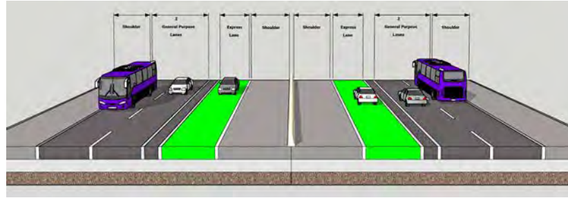
Configuration 2: 2 general purpose lanes, 1 express lane each direction, full inside and outside shoulders
