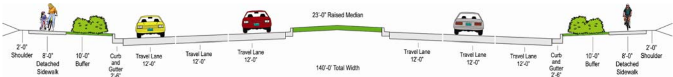
Wadsworth Boulevard Typical Section
