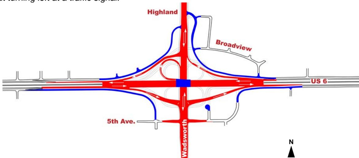
CDOT has identified six travel lanes with a raised median and sidewalks as the proposed design for Wadsworth Boulevard between 4th and 14th Avenues. The basic elements of the design are shown below. CDOT will work with the City of Lakewood on landscaping treatments to create a visually pleasing environment where design and safety standards allow.
