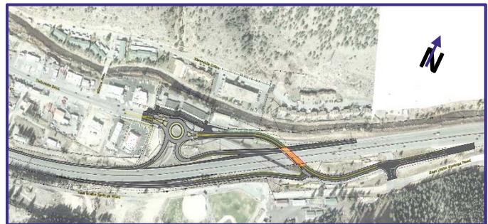
***Work begins in April to build a new bridge over I-70 in the Exit 241 interchange. The current bridge will remain in place for people to use while the new bridge is built immediately east of it and the existing structure will be taken down in the fall. This bridge reconstruction will involve short-term, overnight closures of I-70 for various activities like setting the girders and pouring the deck.***
