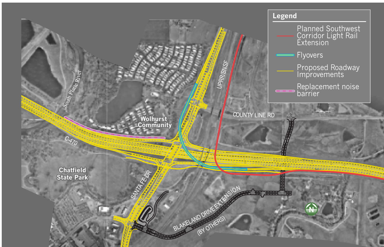
Figure 2-7 Improved Diamond Interchange with Southbound to Eastbound Flyover at Santa Fe Drive
