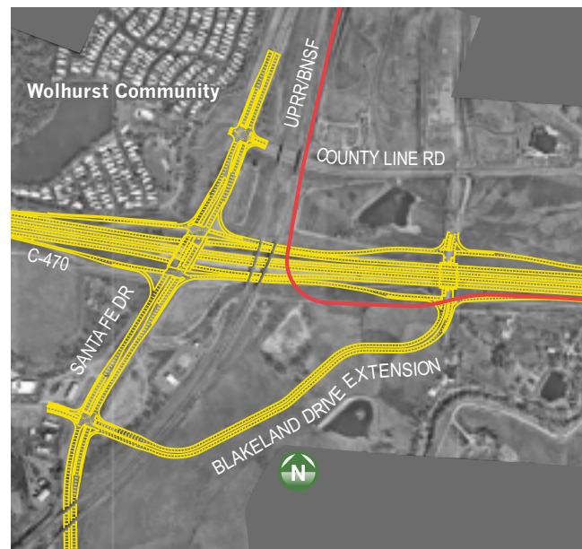
Figure 2-20 Split Diamond Interchange Alternative
