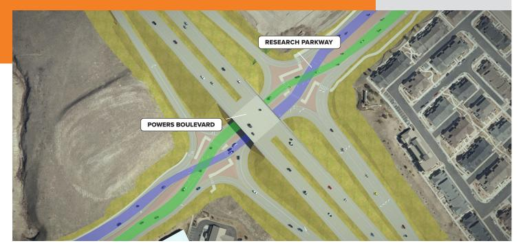
Although DDIs can seem confusing in an aerial view, traveling through them is extremely efficient. Motorists simply follow the pavement markings, signage and traffic signals just like any other intersection.
