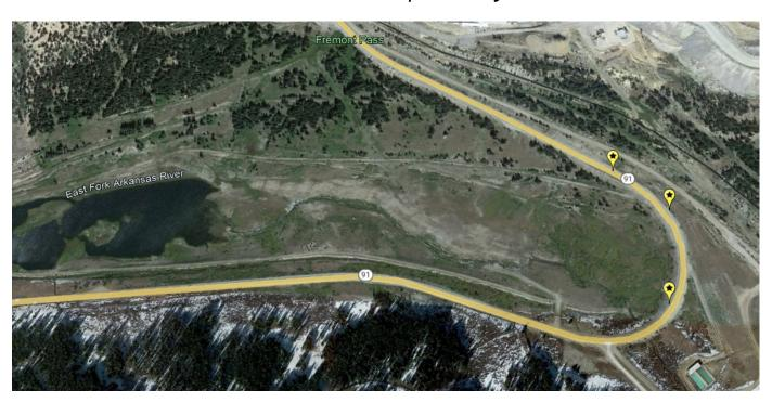
LAKE COUNTY - The Colorado Department of Transportation and American West Construction, LLC will begin work on Monday, June 20 on Colorado Highway 91 to rehabilitate culverts. The culvert at Mile Point 10.52 will be cleaned out and lined and a headwall will also be installed at the outlet structure. The existing pipe at Mile Point 10.70 will be plugged and a new pipe will be installed under CO 91.
