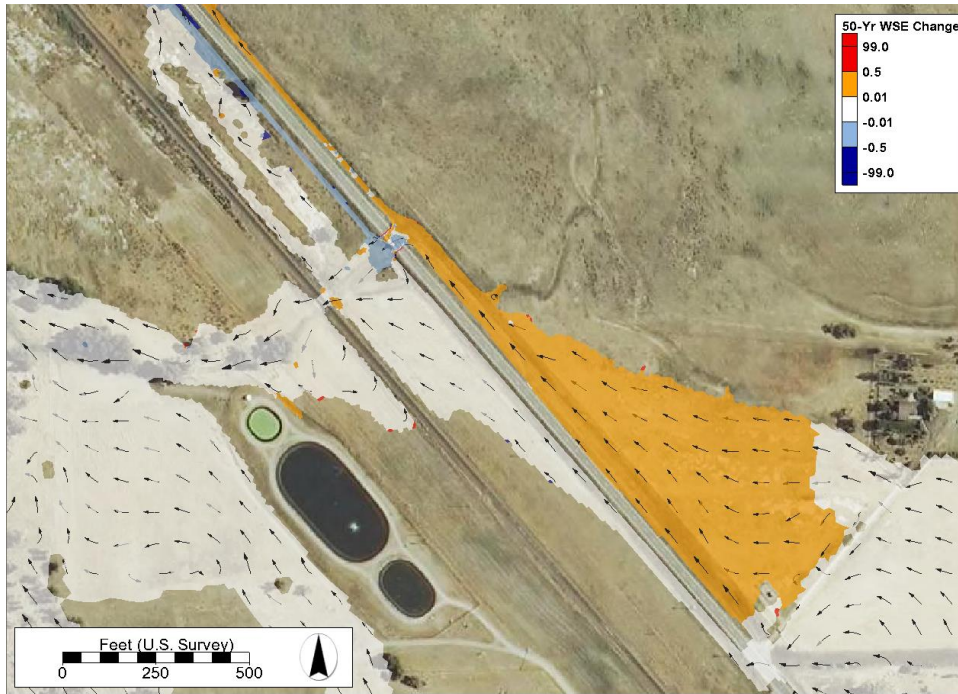
Figure 13: Proposed vs existing WSEL change (orange and red indicate an increase in WSEL) during the 50-year event
