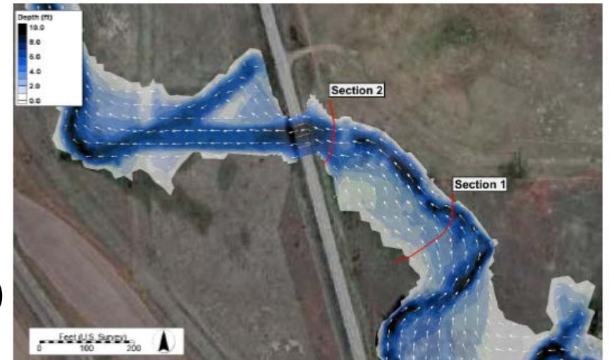
Figure 5: Existing structure G-21-A 100-year depth
