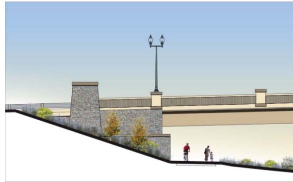
Figure 3.18 – Bridge Monument and Wing Wall
