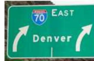
1. Modifications to the I-70 East Denver sign to address the lane assignment change will require a new sign bridge (integral with the proposed retaining wall); the opportunity exists to add the Exit 244 sign to the new sign bridge
