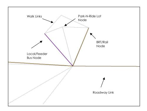
Figure 1: Exploded Node
