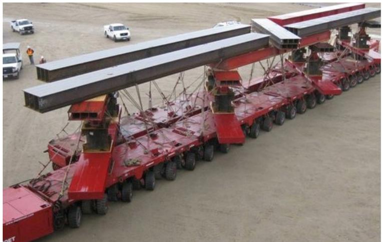
Example of a Self-Propelled Modular Transporters (SPMT)
