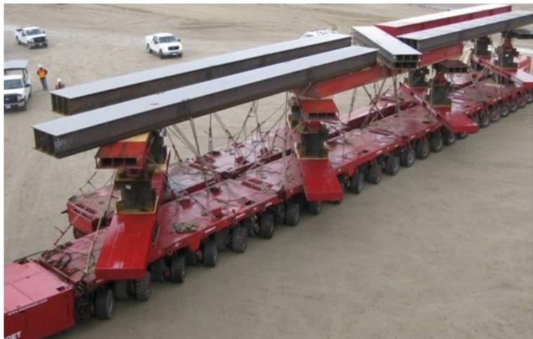
Example of a Self-Propelled Modular Transporters (SPMT)
