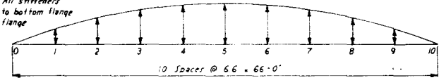
GIRDER CAMBER DIAGRAM SPAN 2 Note: Girder camber diagram above is typical for all girders in span 2. Cut girder web to camber, as shown on bottom line of table below. Slab remains constant 7 1/2" thick
