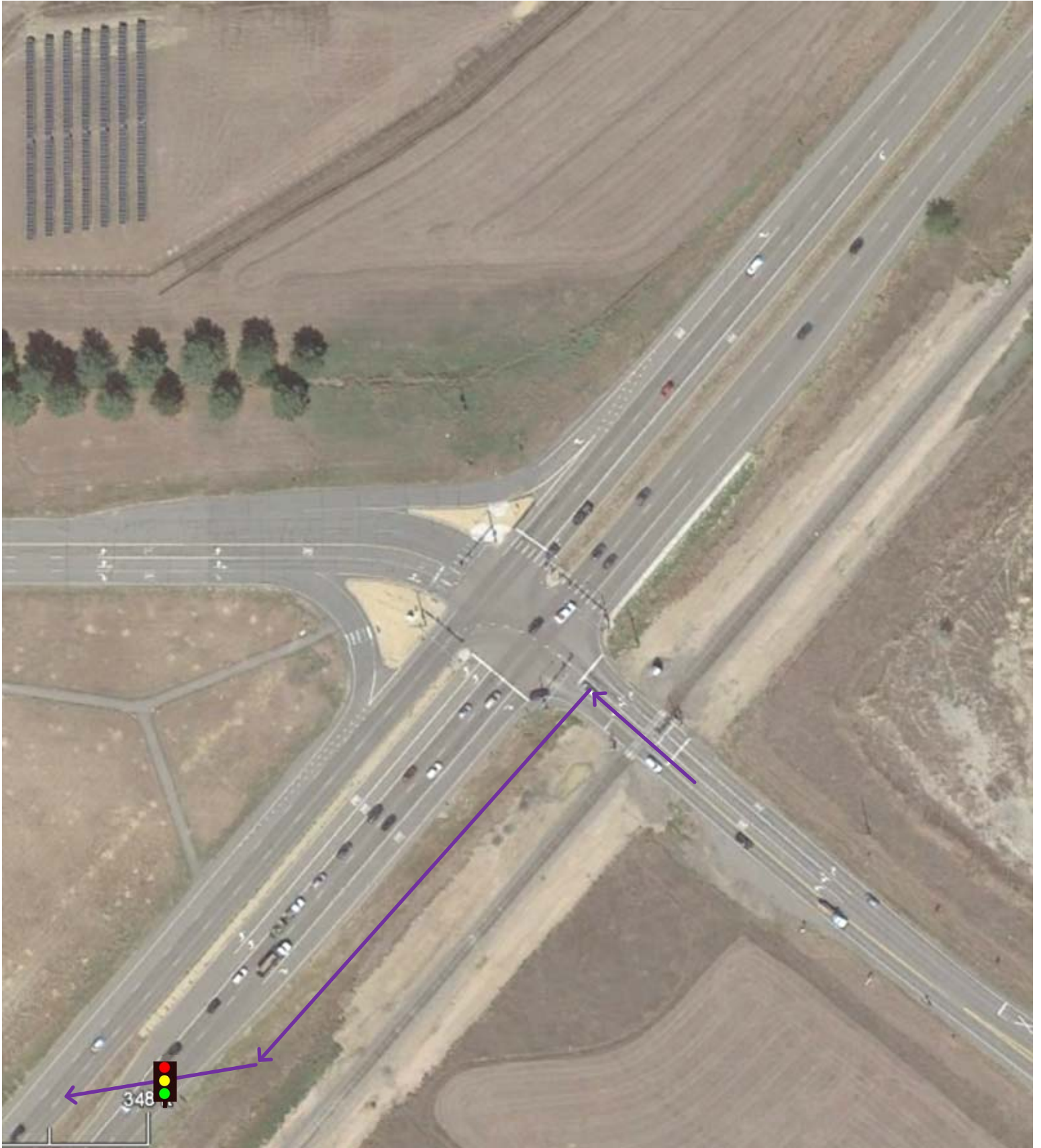
SH 119 & SH 52 Continuous Flow Intersection (CFI)
