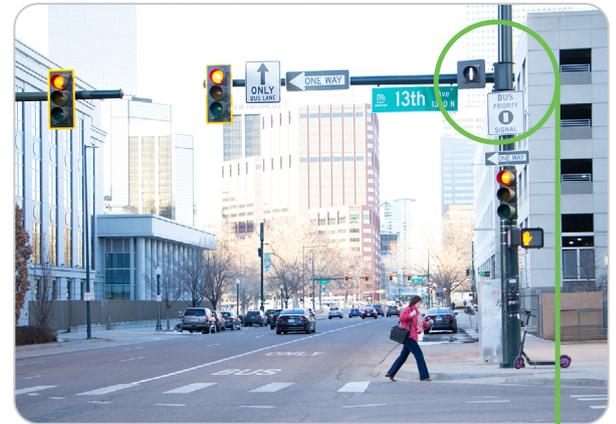
A special signal with a vertical line tells buses to proceed through the intersection while general traffic waits at the red light
