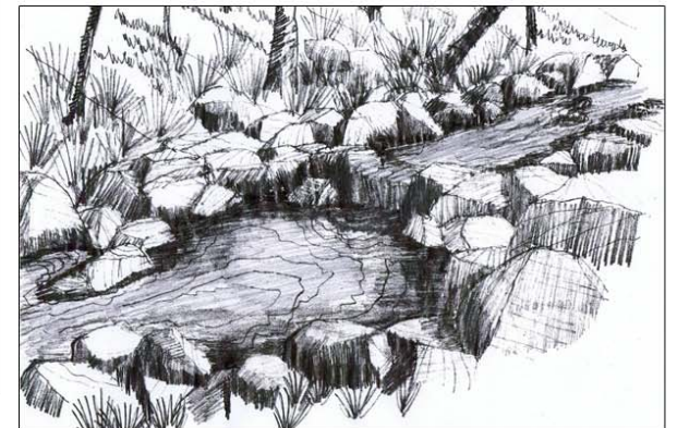
D | Drop structure using indigenous rock construction.
