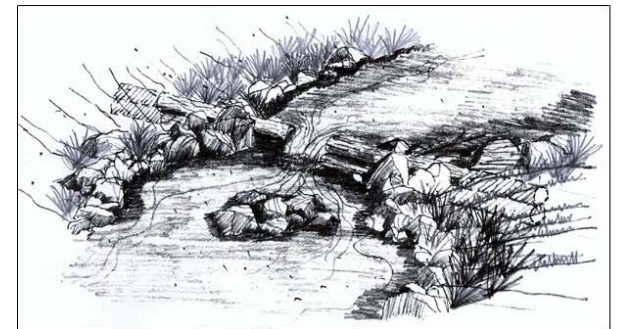
C | Drop structure using indigenous log construction.
