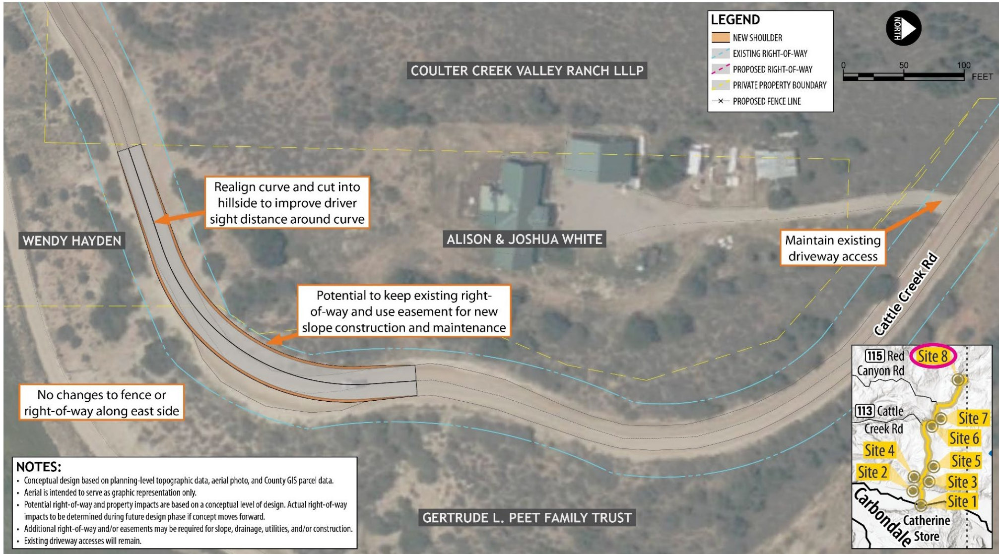
Figure 11. Garfield County Site 8 - Hillside Grading
