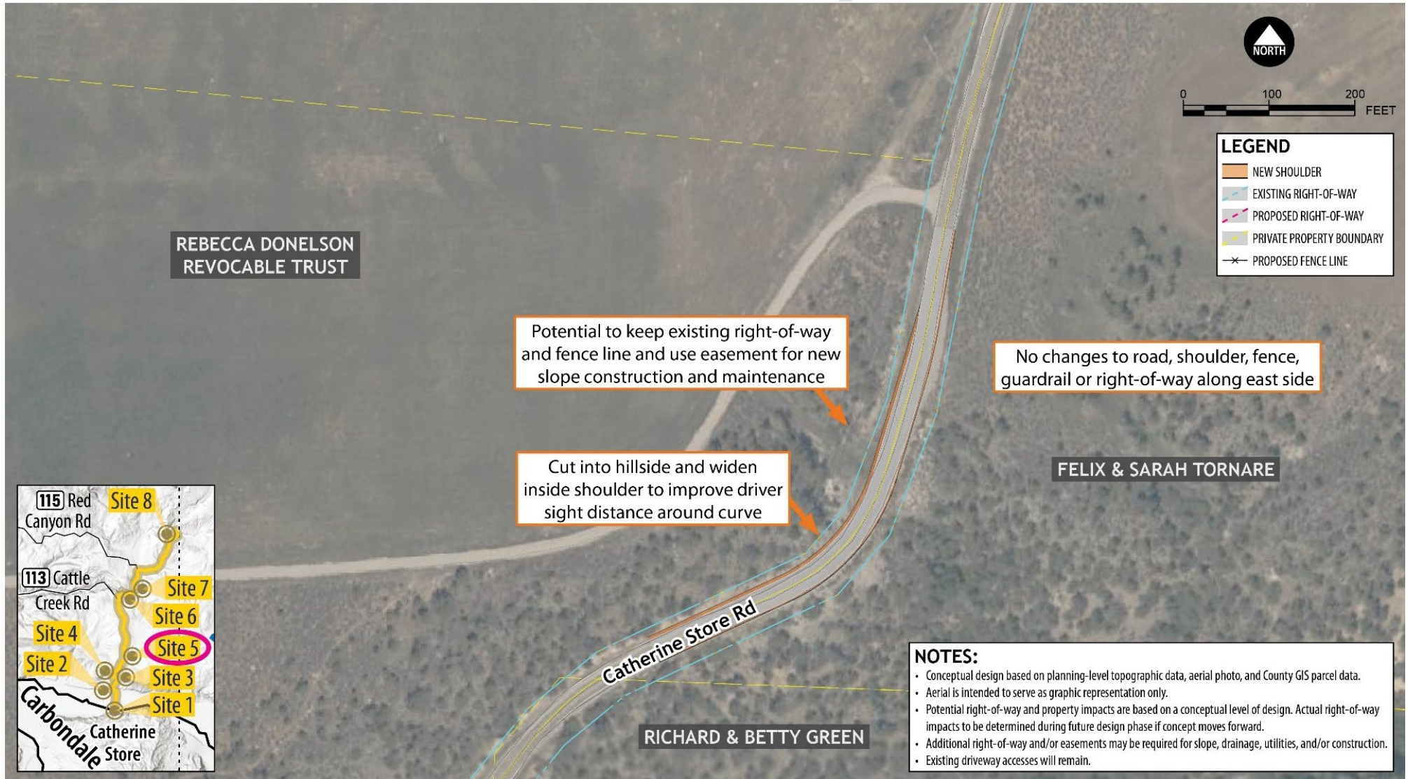
Figure 7. Garfield County Site 5 - Hillside Grading
