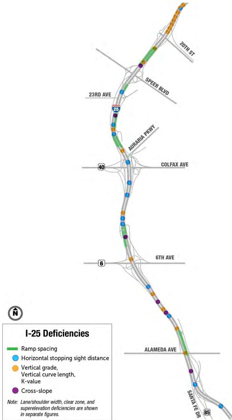
**Figure 2. Ramp Existing Geometric Deficiencies (20th Street to Santa Fe Drive)**
