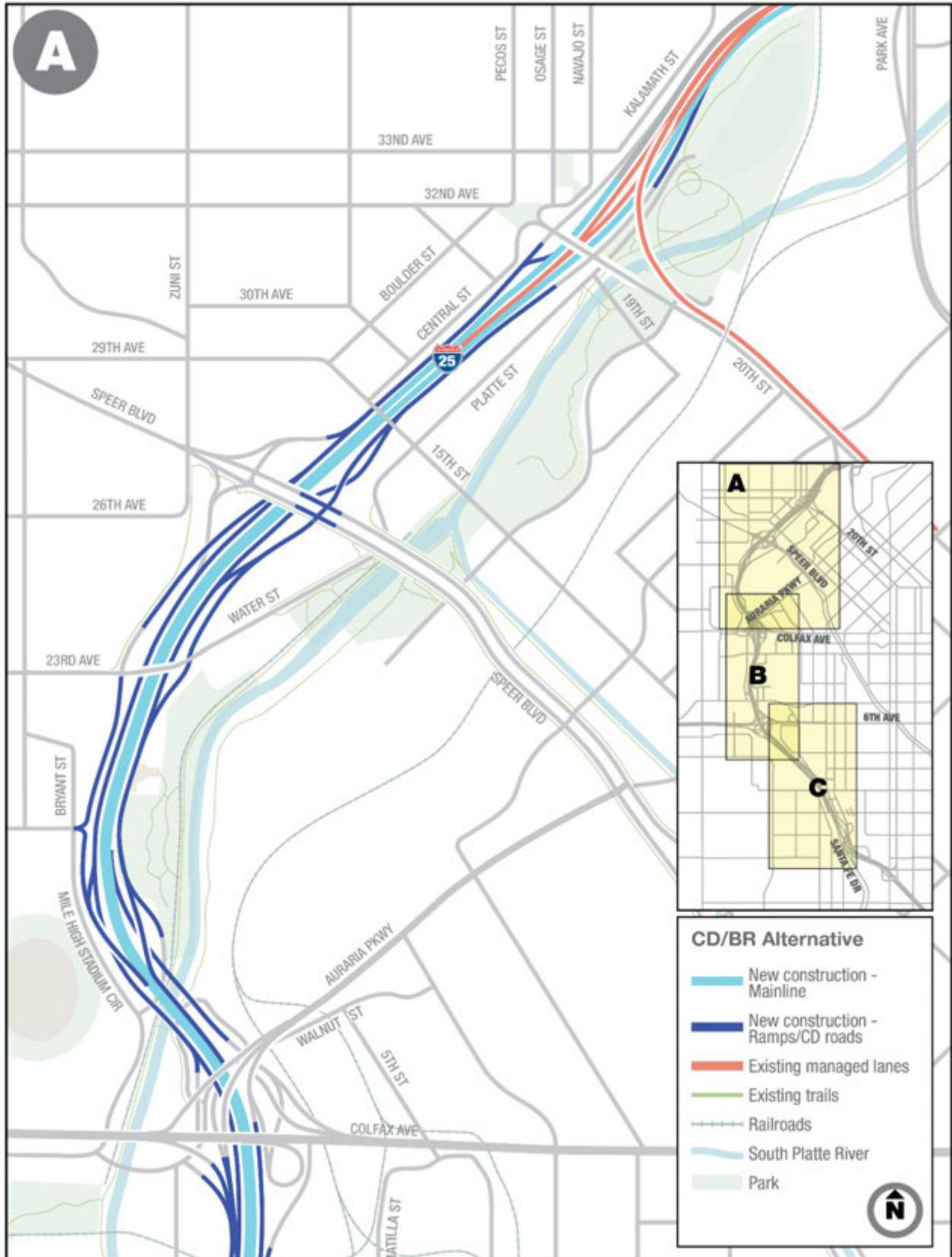
Figure 23 Collector/Distributor Roads and Braided Ramps Alternative (Continued)
