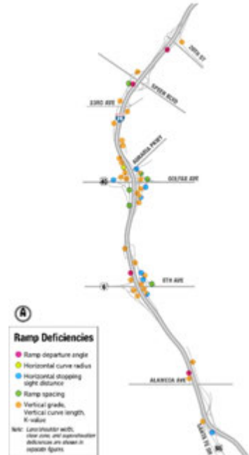
Ramps are too close together and have tight curves
