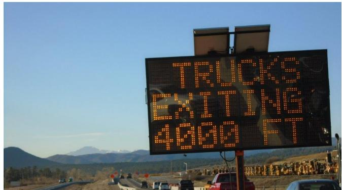
farther back in the corridor is triggered and will light up a sign to warn motorists in time to slow down and yield to the truck.
