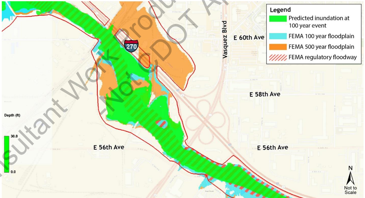
Figure 13. Overlay of Model Inundation Extents between Vasquez Boulevard and Brighton Boulevard with FEMA Flood Zones Source: Jacobs
