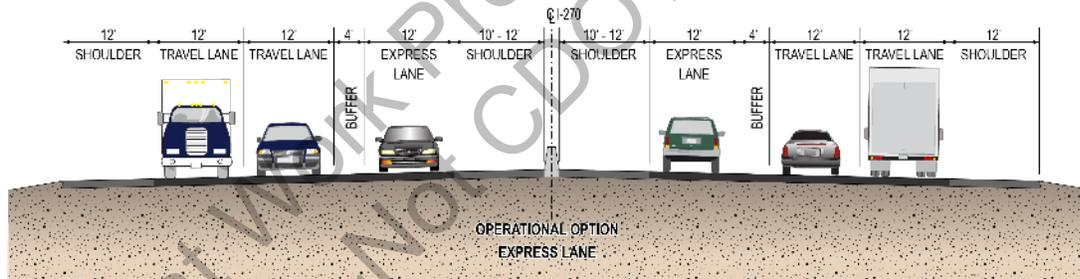
Figure 2-1. Typical Roadway Section without Auxiliary Lane
