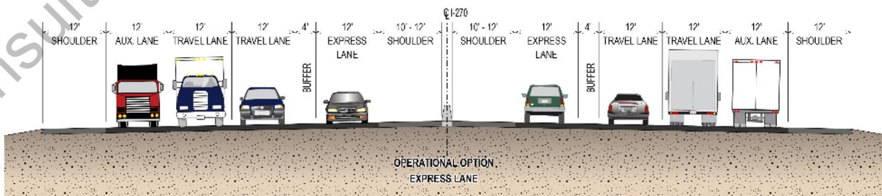
Figure 2-2. Typical Roadway Section with Auxiliary Lane
