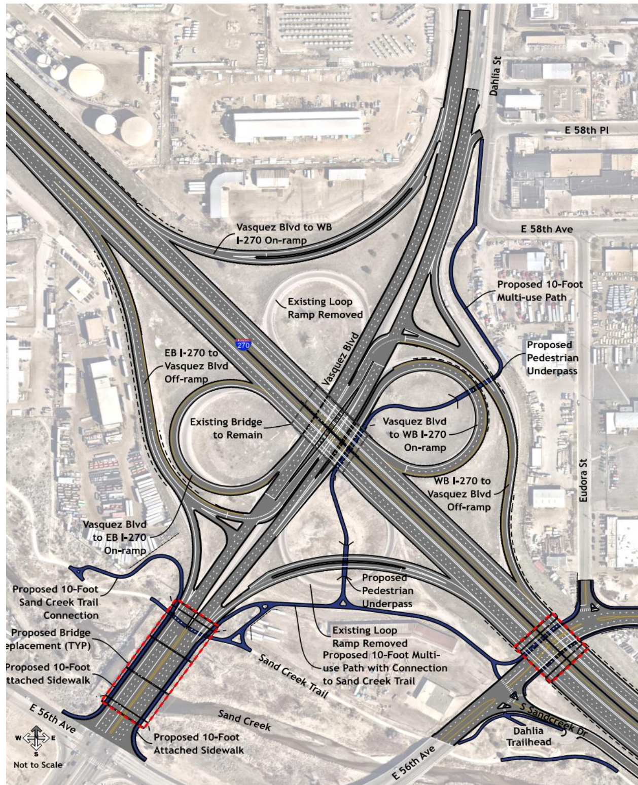
Figure 28. Vasquez Boulevard Crossing under I-270 Design
