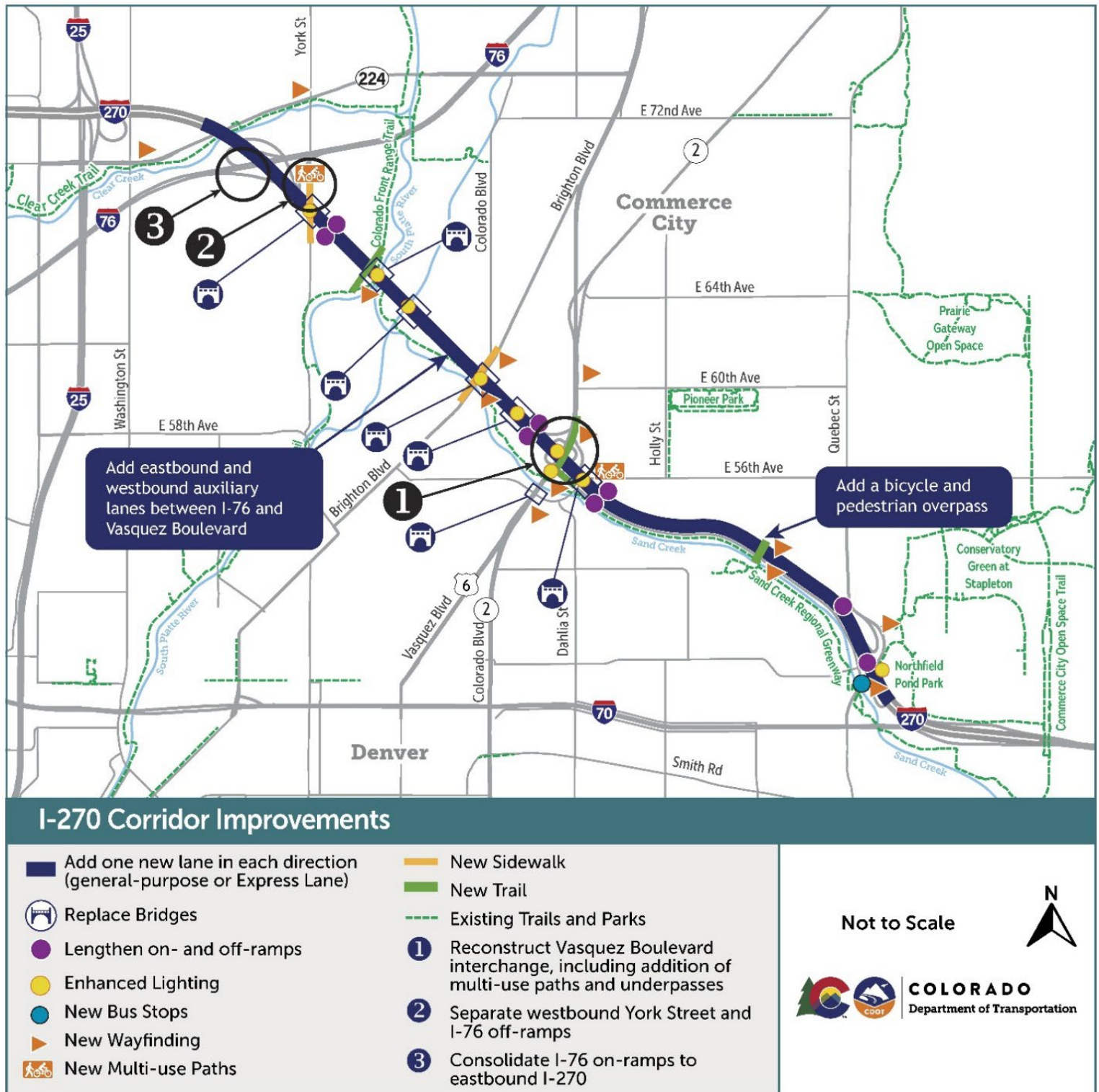
Figure 3-3. Improvements Included in Both Build Alternatives
