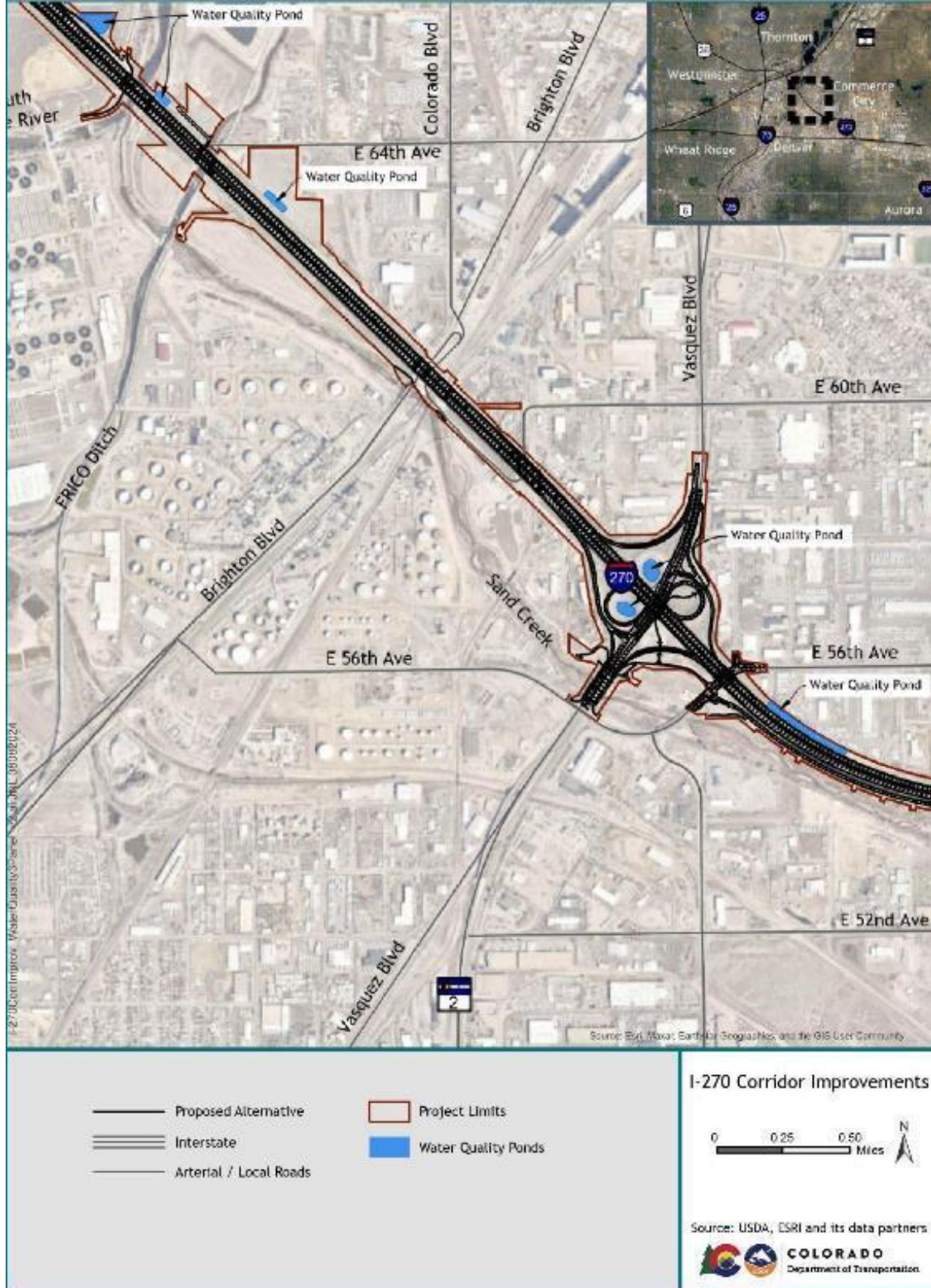
Figure 12. PWQ Locations for Build Alternatives (Central Section)
