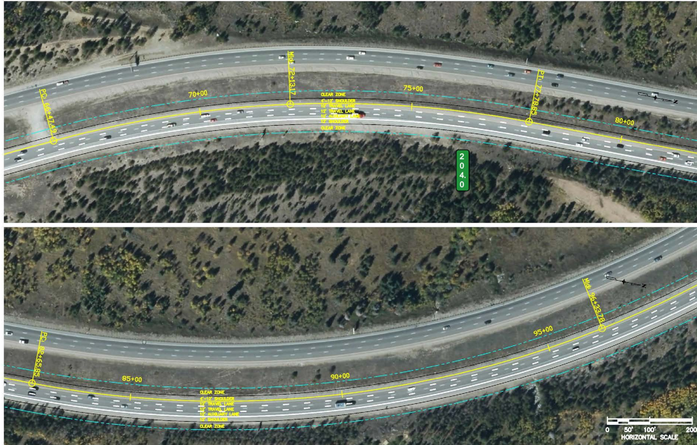
Figure 5-2: I-70 Eastbound Auxiliary Lane Concept (Exit 203-205) CONTINUED
