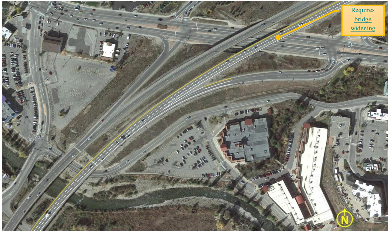
Figure 5-5: Modified I-70 Eastbound Lane Balance at Exit 205 – Exit Lane Developed on Ramp
