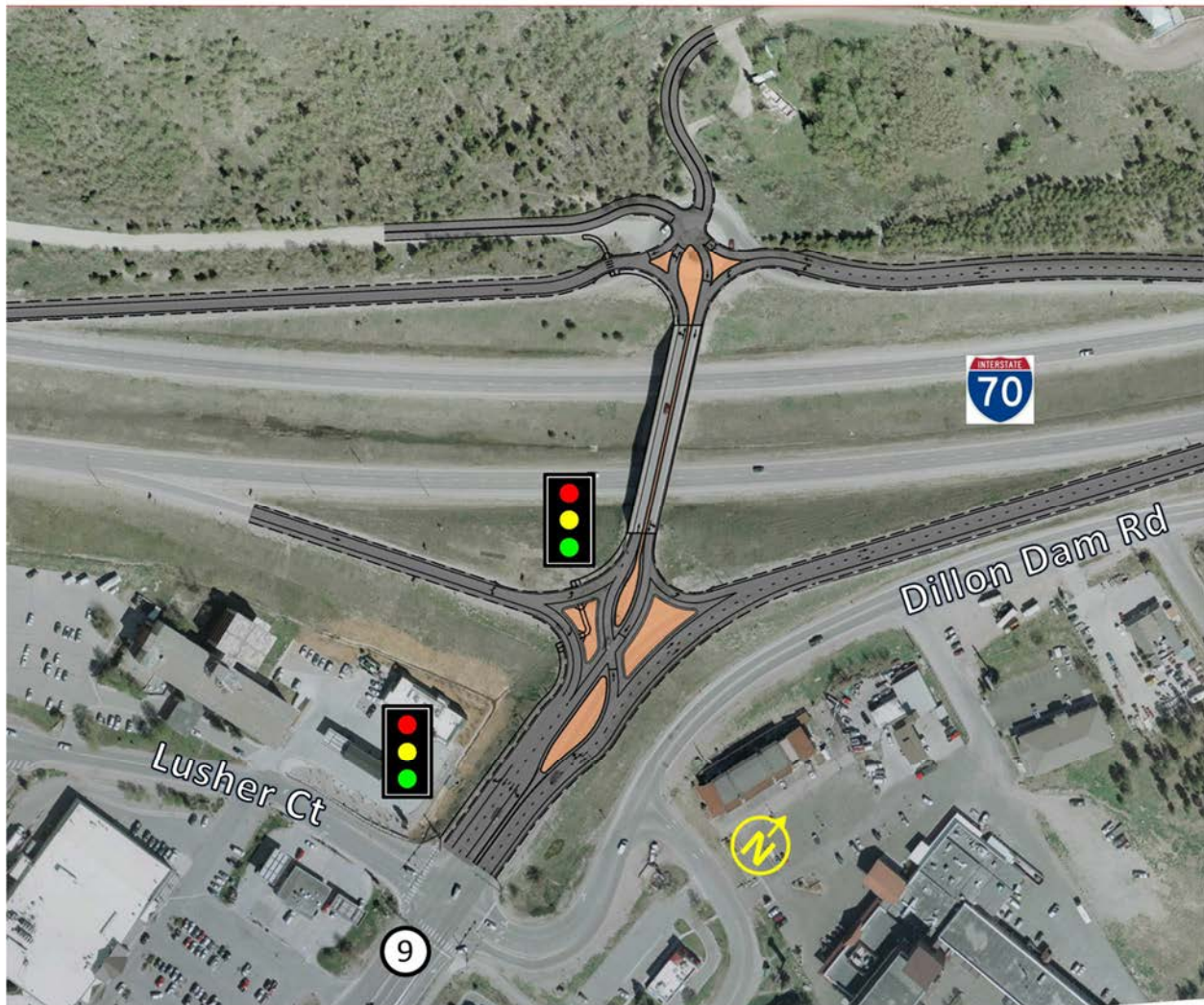
Figure 5-11. Exit 203 Diverging Diamond Interchange
