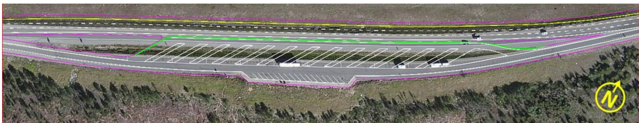
Figure 5-8: Diagonal Parking Scenic Overlook/Chain-up Station Layout
