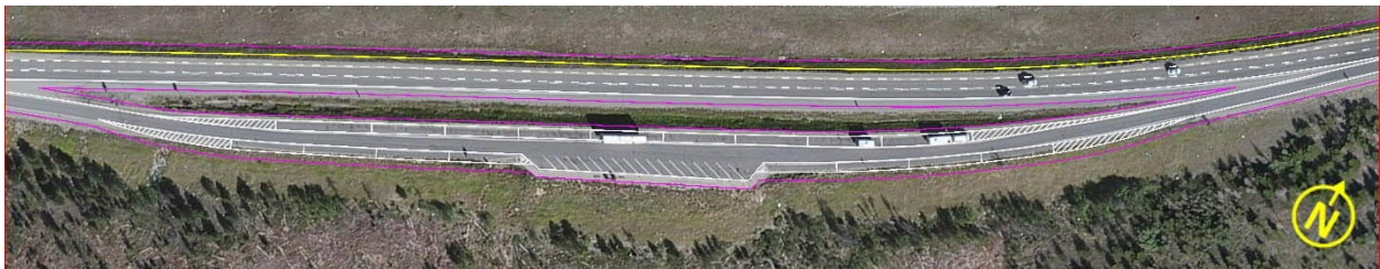
Figure 5-6: Modified Existing Scenic Overlook/Chain-up Station Layout
