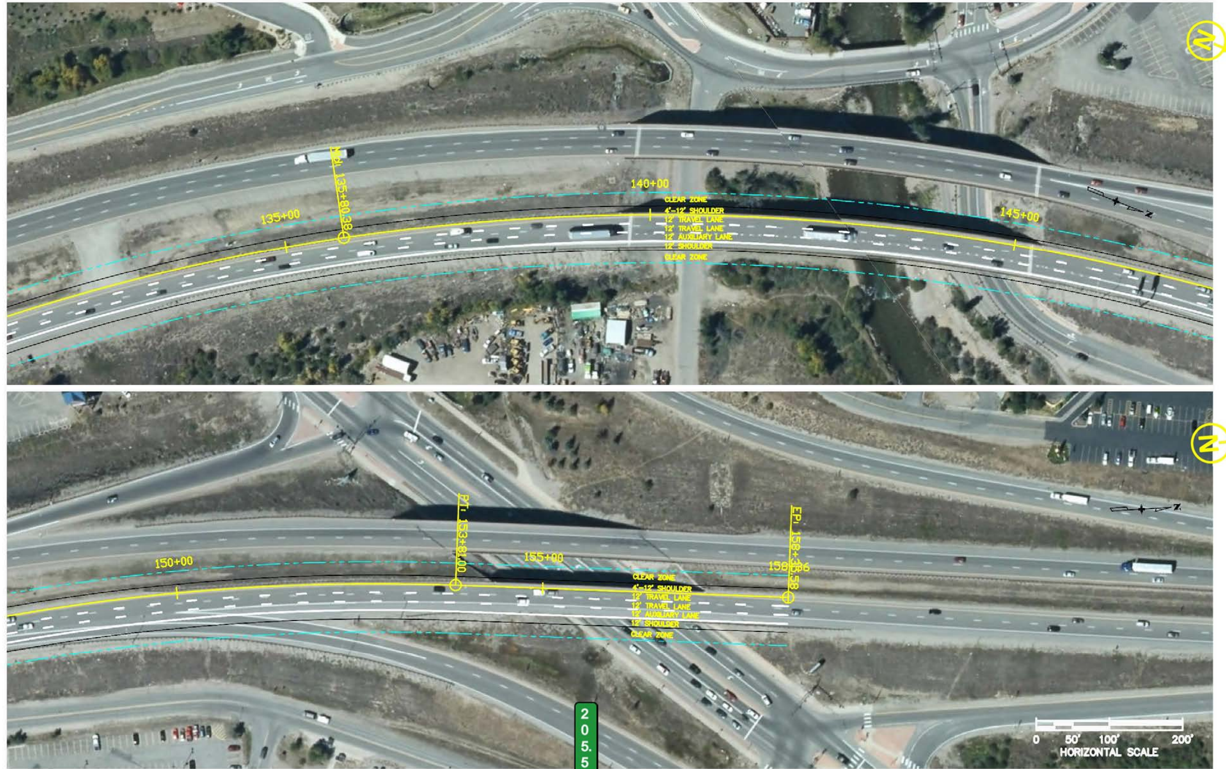
Figure 5-2: I-70 Eastbound Auxiliary Lane Concept (Exit 203-205) CONTINUED
