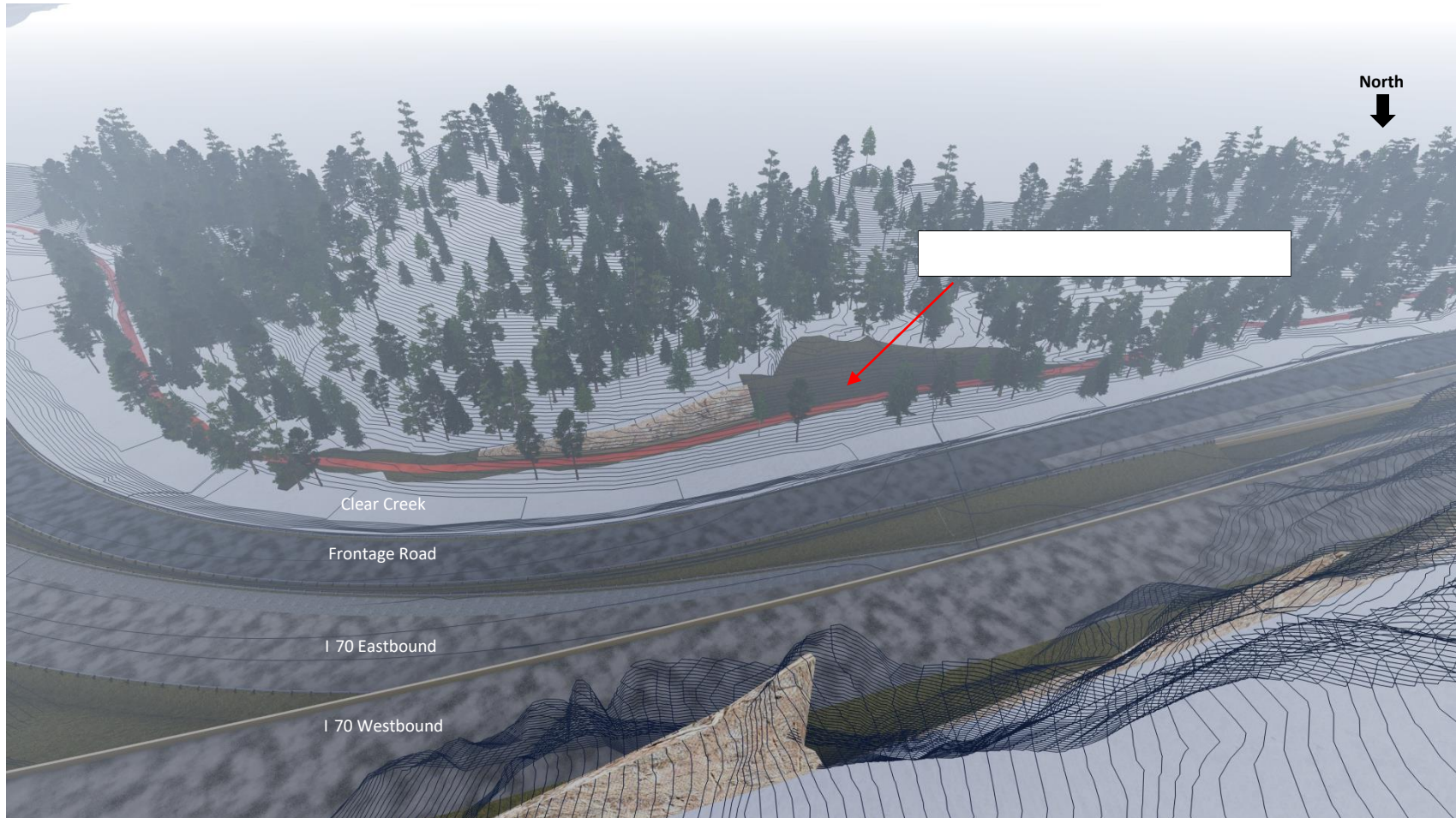
Figure C-1. Proposed Rock cuts for ADA Slope Compliance, Scott Lancaster Memorial Trail, Tunnel Alternative, North Frontage Road Option
