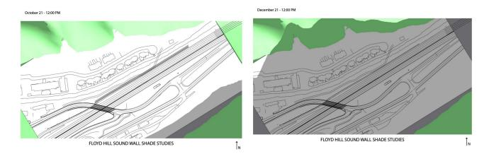
The renderings show that shade from the Sound Wall is negligible through most of the winter months due to the large shadow of the Mountain. During Oct, Feb, and March, the wall shades more of the trail than would be shaded by Mountain shadow. Regardless of the Sound Wall, a long term maintenance plan will be necessary to ensure ice is not an issue on this section of the trail.
