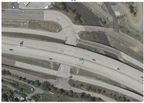
The plan is to join these two parallel roads to reduce this intersection confusion. This will also streamline the necessary bridge repair (current bridges are hydraulically compromised), replacing two old bridges with one improved bridge (Bridge Q).
