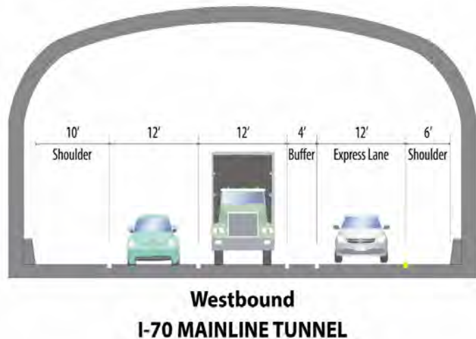
Exhibit 25. I-70 Westbound Tunnel Typical Section
