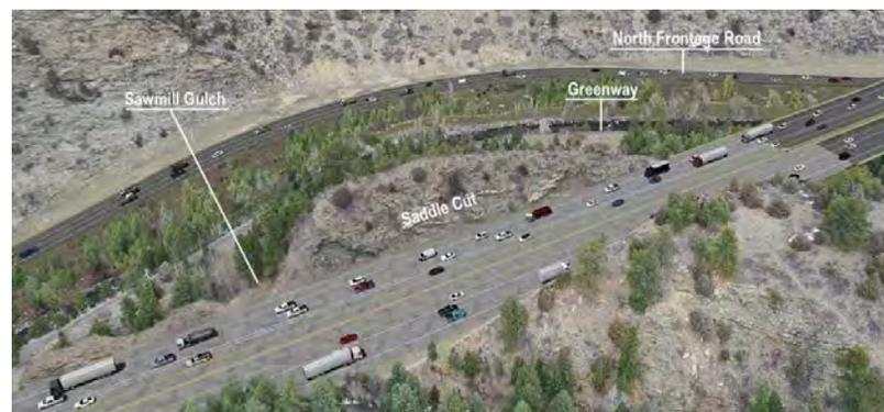
The Canyon Viaduct Alternative would reconstruct the US 6/I-70 interchange. The reconstructed interchange would add a new on-ramp for US 6 to eastbound I-70, which does not currently exist, and would modify the on-ramp for US 6 to westbound I-70 from a left-lane entrance to a traditional right-lane entrance. The eastbound I-70 off-ramp to US 6 would be removed, and this movement would be provided through the Hidden Valley/Central City interchange and new frontage road.
