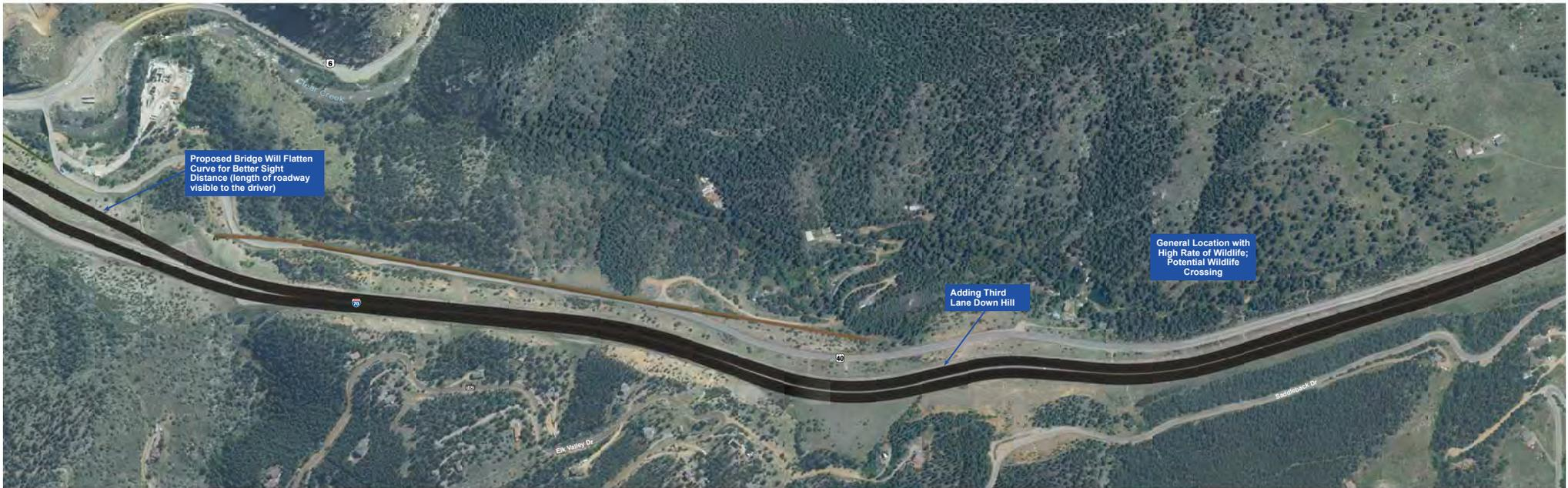
Proposed Bridge Will Flatten Curve for Better Sight Distance (length of roadway visible to the driver)
