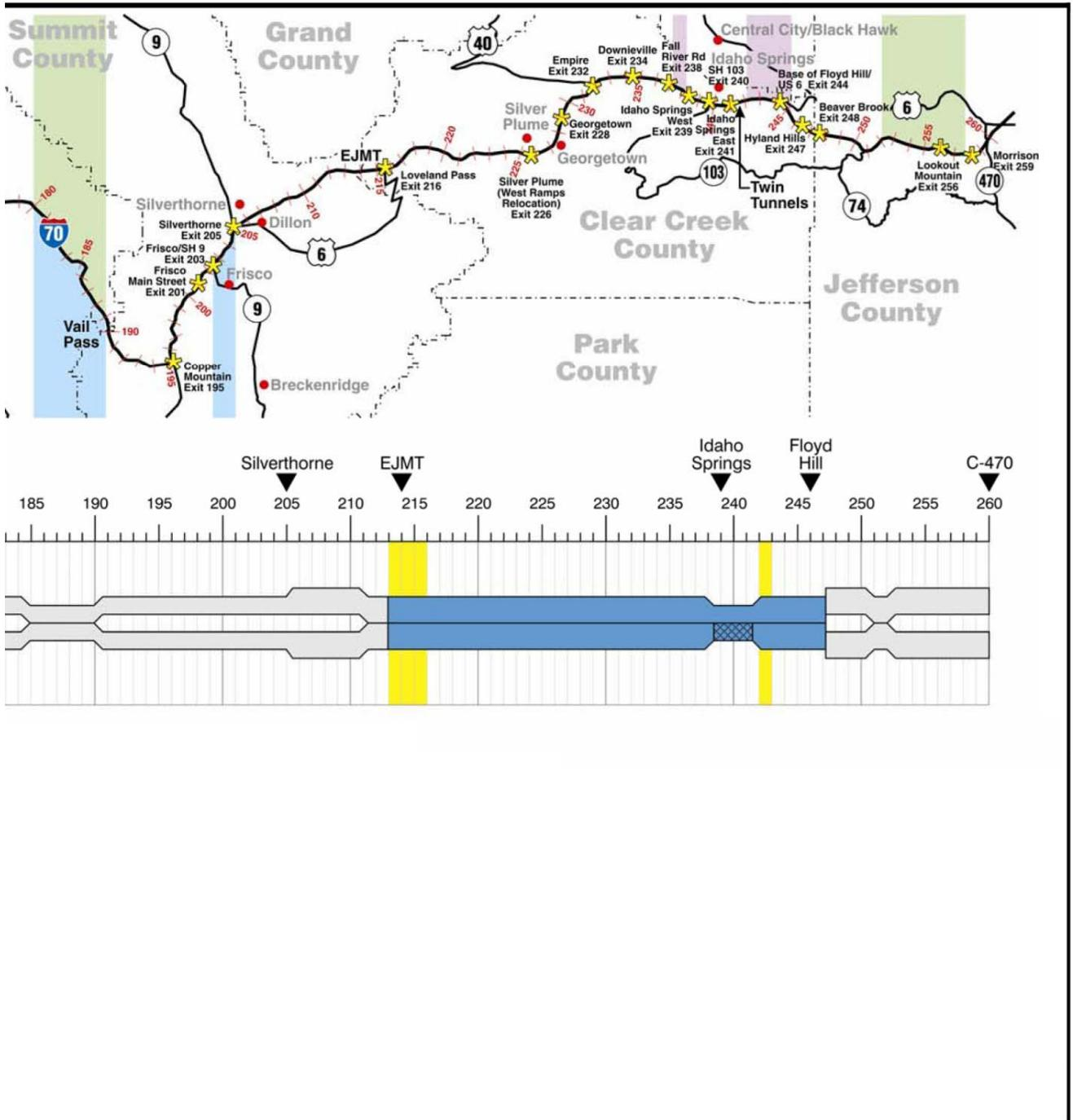
Figure 23. Six-Lane Highway 55 mph Alternative Typical Configuration and Structured Configuration in Idaho Springs
