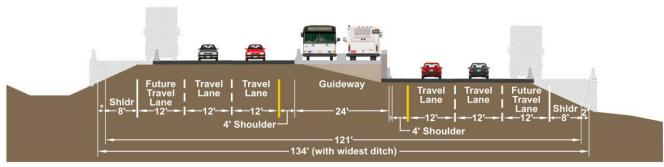
Figure 39. Bus in Guideway with Highway Preservation
