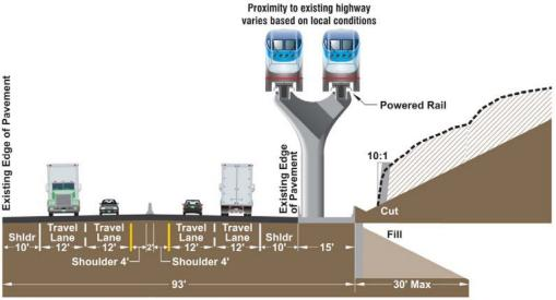
Figure 13. Advanced Guideway System Typical Configuration
