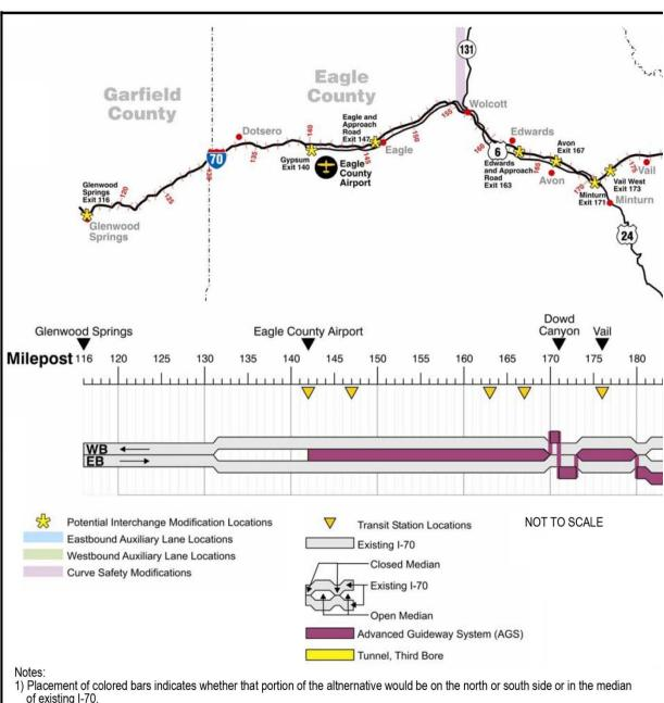
Figure 12. Advanced Guideway System Alternative Overview
