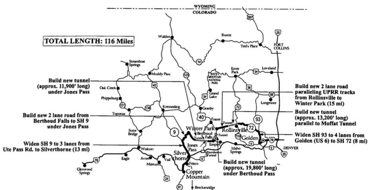
Figure 8. Alternate Route 5 – Denver to Copper Mountain via Moffat, Berthoud Pass, and Jones Pass Tunnels (SH 72/SH 9)
