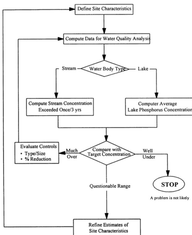
The input parameters required in the model include drainage areas, stream flow for the watershed, rainfall characteristics, pollutant concentrations in the runoff, and instream target concentrations to be used for comparison of exceedance frequency. The model outputs are frequency of storm events exceeding specified target concentrations and once in 3-year stream concentrations.
