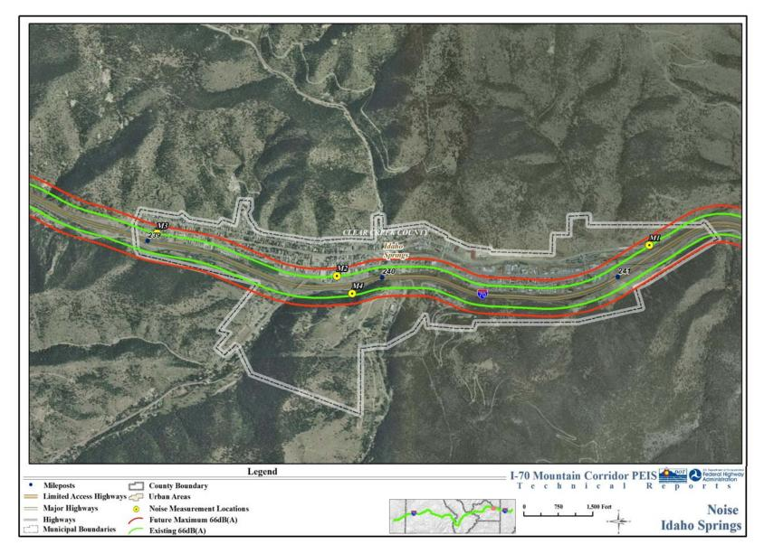
Figure 12. Idaho Springs 66 dB(A) Noise Contours and Measurement Locations
