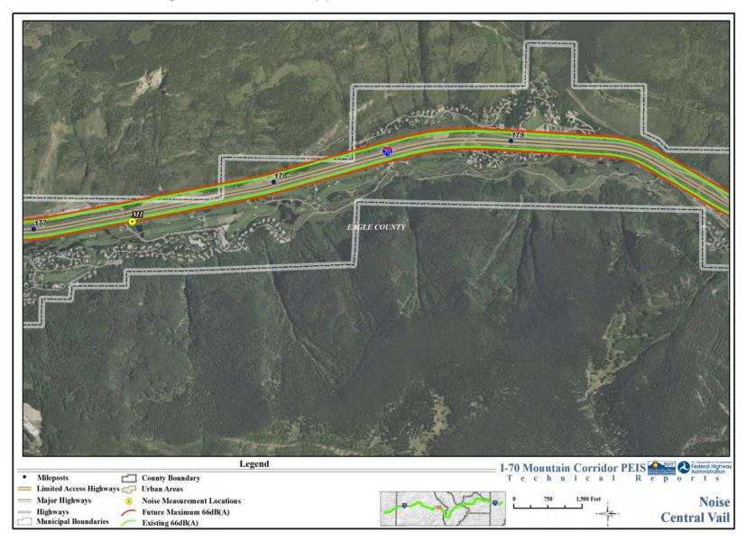
Figure 3. Central Vail 66 dB(A) Noise Contours and Measurement Locations
