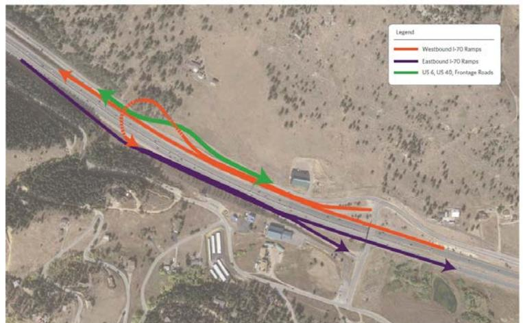
The Close Interchange at US 6 (move to top of Floyd Hill) concept, pictured above, closes the US 6 interchange and moves it to the top of Floyd Hill. Traffic from US 6 will need to go back up the hill. This option does not appear to be optimal for trucks or community. Intersections at both ends will be modified.
